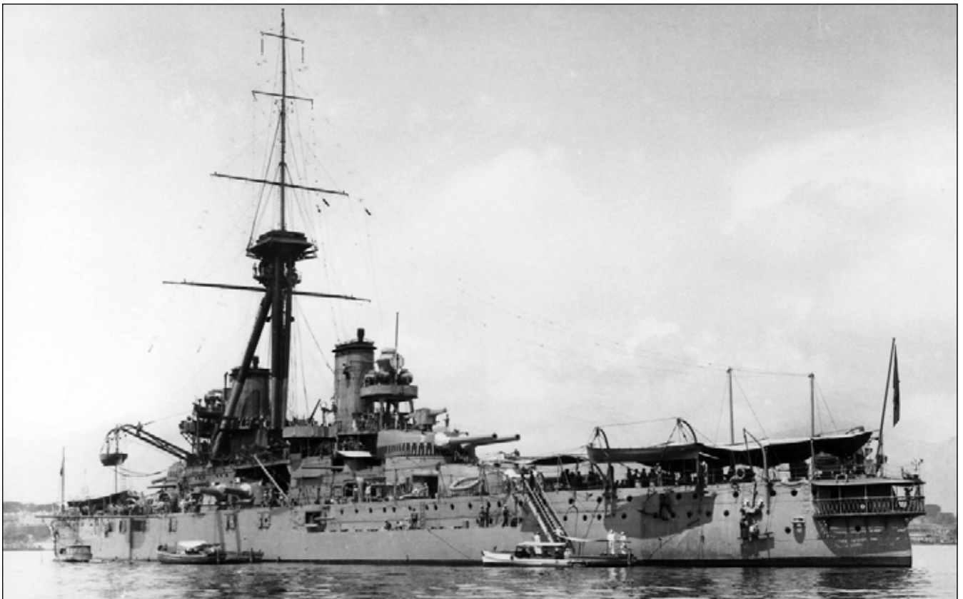
23 The Brazilian battleship Minas Geraes which inspired the STT/Popper design No V armed with twelve 30.5 cm/45 guns
