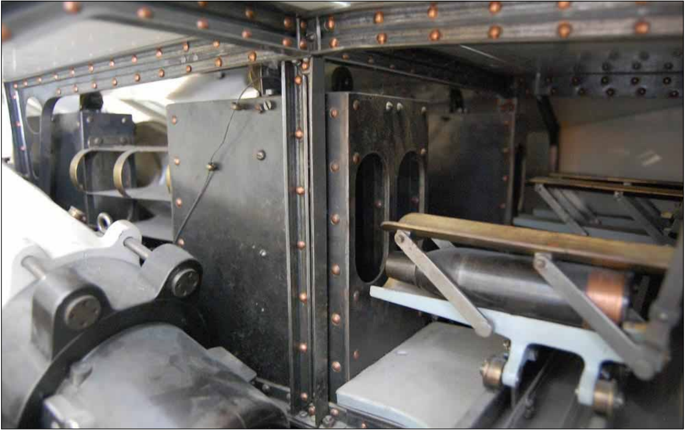
26 The 30.5 cm/45 triple turret model made by Škoda. Note the projectile with AP cap but without ballistic cap on the loading car. Note also the connecting trays between the main and the auxiliary ammunition hoists
