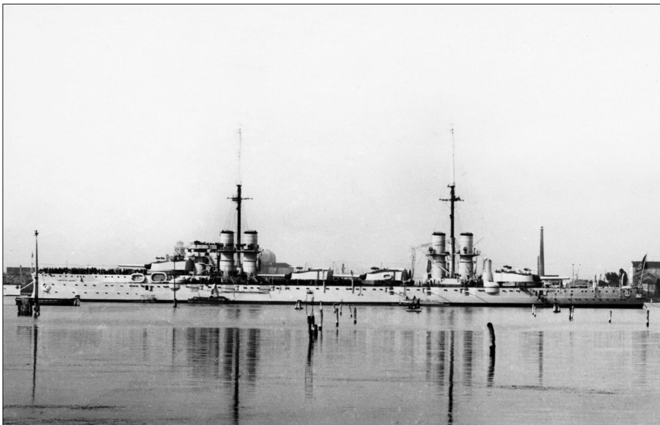
29 The first Italian dreadnought, the Dante Alighieri armed with twelve 30.5 cm/46 guns in four triple turrets
